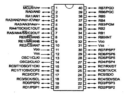
Figure 1: Pin diagram of PIC16F877A microcontroller
