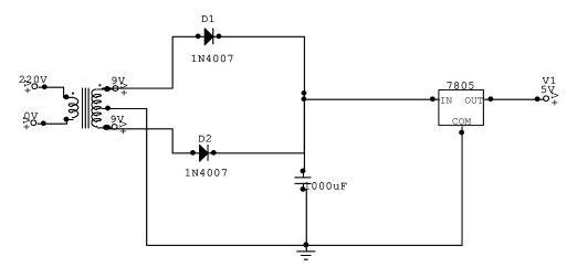
Figure 6: Constructed circuit diagram of +5V regulated power supplies
