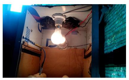
Figure 11: Photograph of setting bulbs and fans in the incubator model.
