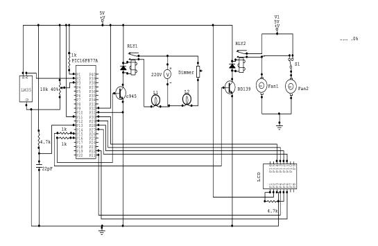
Figure 7: The constructed controlled circuit of hen egg incubator model
