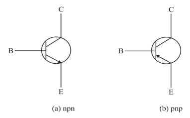
Figure 2: Standard bipolar junction transisor (BJT) symbols
