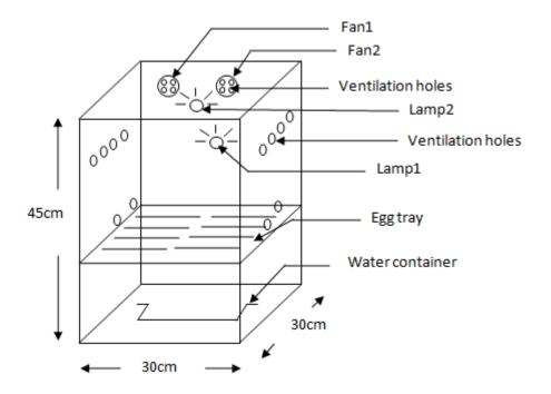
Figure 5: Dimension of constructed hen incubator model
